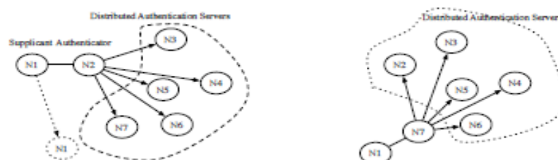
Fig 2: Fantacci's Distributed Node Authentication Model (a) Initial authentication by 2 N (b) 1 N reauthenticated by 7 N
